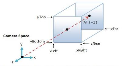
**Orthographic Projection:** Camera positioned infinitely far away at  $z = \infty$
