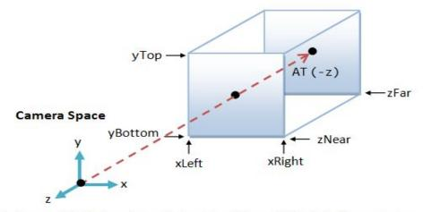
**Orthographic Projection:** Camera positioned infinitely far away at  $z = \infty$
