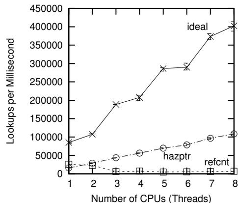
**Figure 9.3:** Pre-BSD Routing Table Protected by Hazard Pointers
