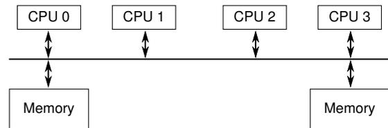
**Figure 15.7:** Global System Bus And Multi-Copy Atomicity
