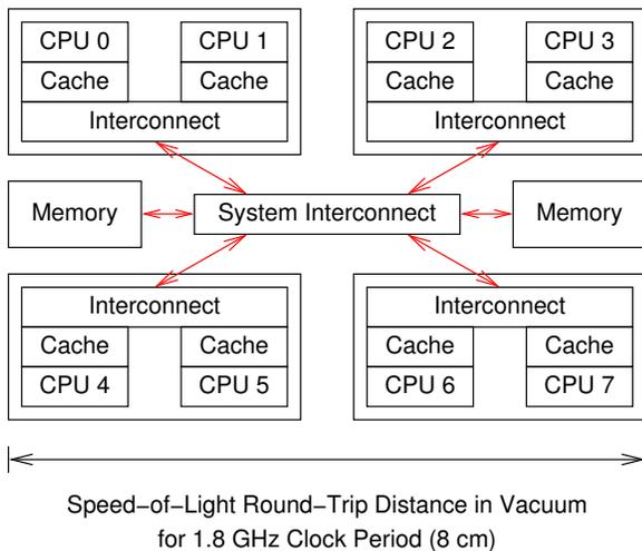
Figure 3.9: System Hardware Architecture
