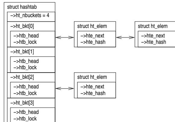
**Figure 10.1:** Hash-Table Data-Structure Diagram**Listing 10.2:** Hash-Table Mapping and Locking
