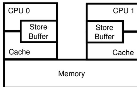
**Figure 15.1:** System Architecture With Store Buffers
