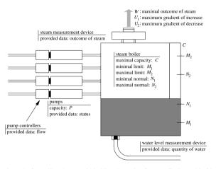
Mickael Kerboeuf et al: Specification and Verification of a Steam-Boiler with Signal-Coq, 2010
