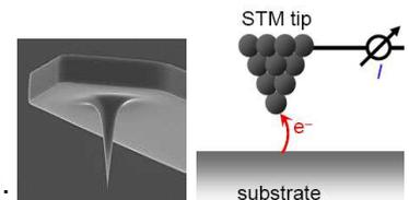
(B) **Proximal Probes:** Optical fibers, STM/AFM probe tips that are scanned in close proximity over the sample surface. Small excitation energies and excitation volume.
