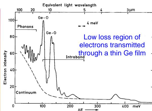
Fig. 5.7. Energy-loss spectrum of an evaporated Ge film due to phonons
